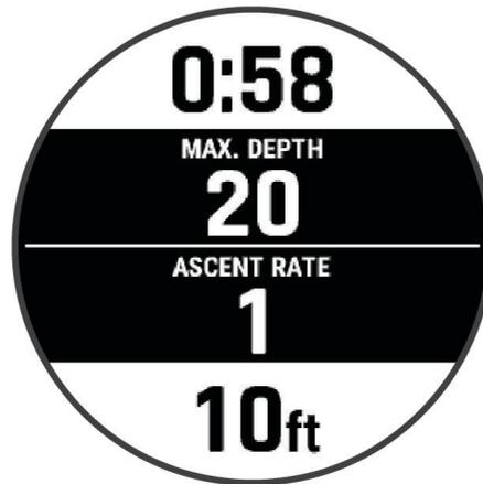
**In-dive screen:** Displays the information about the current dive, including the elapsed time, current and maximum depth, and rate ascent or descent. You can edit the data screen layout and data fields (*Customizing the Data Screens*, page 105).
