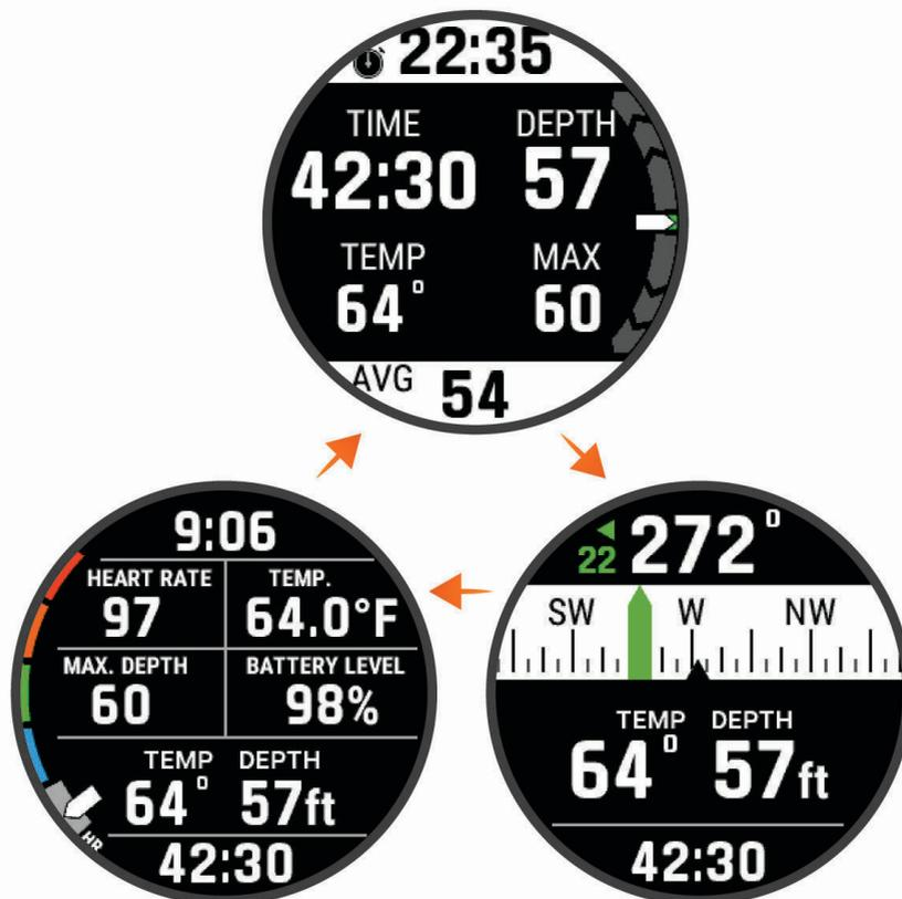
**Dive stopwatch:** Displays the bottom time stopwatch; current, maximum, and average depth; and rate of ascent or descent (*Using the Gauge Dive Stopwatch*, page 18).
