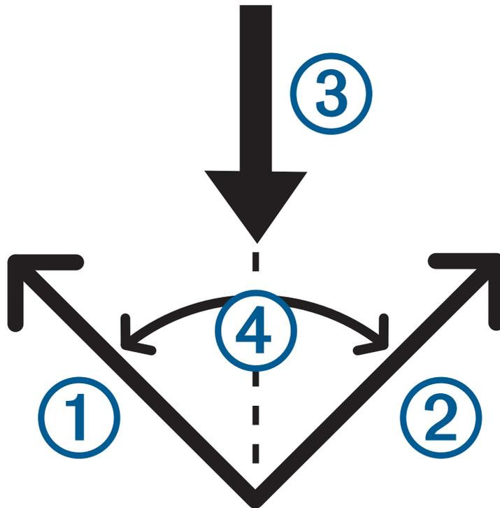
The device uses this data to determine whether your boat is being lifted or headed due to wind shifts.
