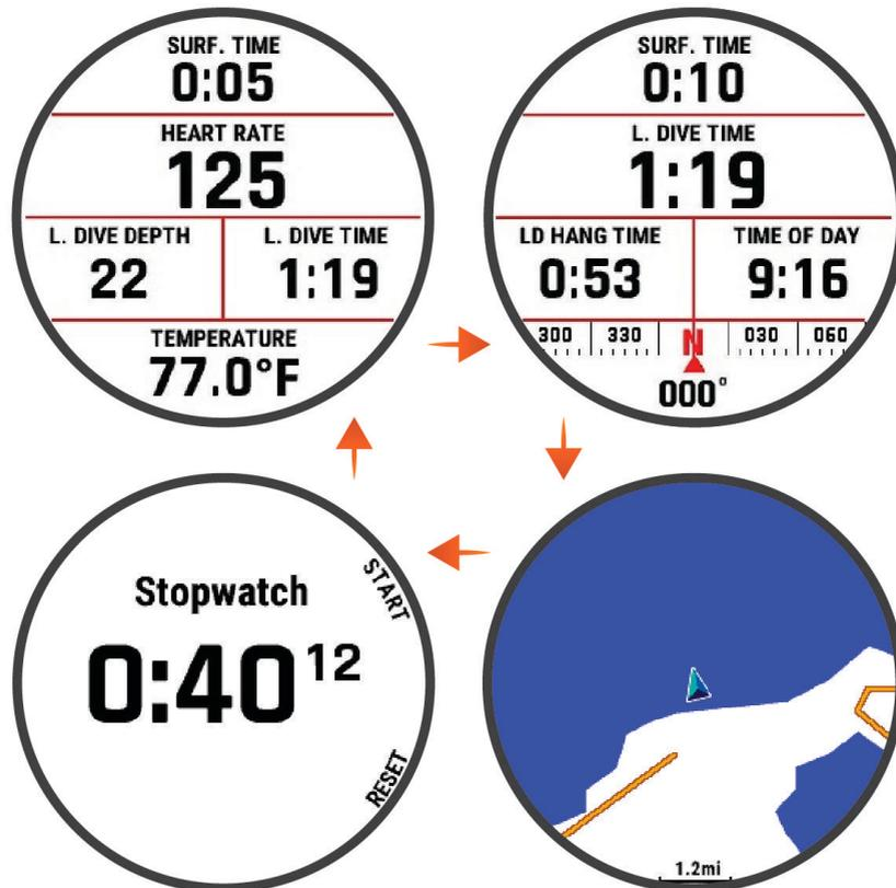
**Surface interval screen 1:** Displays the current surface interval time, heart rate, and last dive information. You can edit the data screen layout and data fields.
